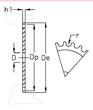
C = 1 D = 20 De = 192.1 Dp = 188.06 For chain size = 3/8 x 7/32 For chain type = 06 B-1 h1 = 5.3 Solution Number of teeth = 62
